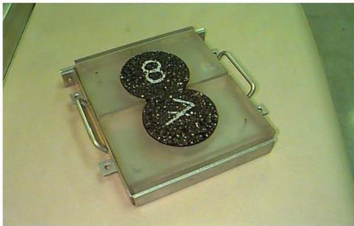
Figure 1—Cylindrical Specimen Mounting System
