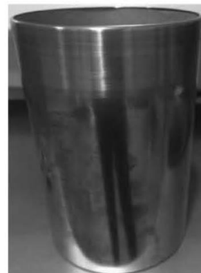
FIG. 3 Centrifuge Cup with Inlay Paper
